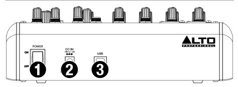
1. Power Switch: Flip this switch to power TrueMix 600 on and off.
