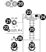
**Note:** Most dynamic microphones do not require phantom power, while most condenser microphones do. Please use caution and consult your microphone's documentation to find out if it requires phantom power **before** connecting your microphone to the **Mic Inputs** and attempting to use this function. Misapplication of this function can damage certain types of microphones, such as ribbon microphones. Always connect the microphone FIRST, then turn on phantom power.
