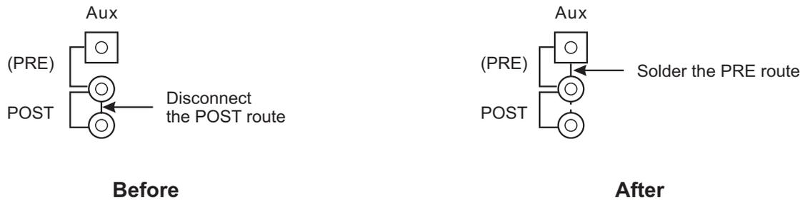
**Modification on mono and stereo channels**
