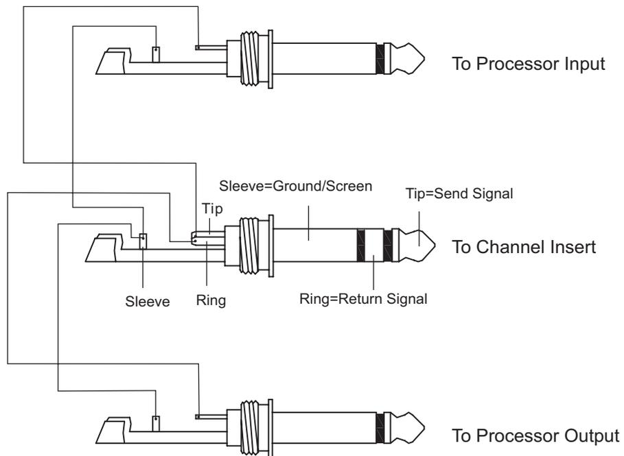
**Y-Stereo lead for insert Connection**
