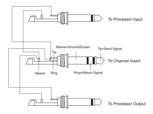
Y-Stereo lead for insert Connection
