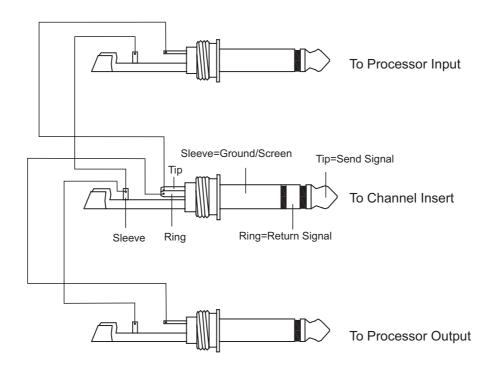
Y-Stereo lead for insert Connection
