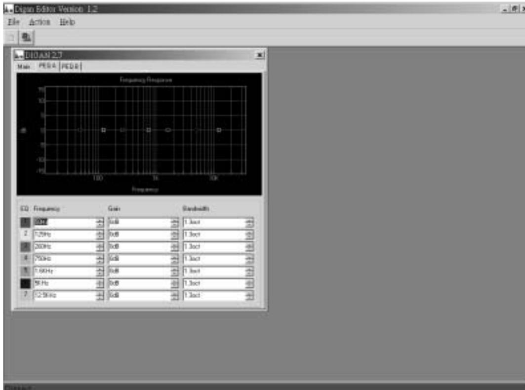
When you go to parameter equalizer, the PC will display above picture, you can adjust the frequency, gain, and bandwidth according to the application. If this unit is in LINK function, the change on channel A will be applied to channel B also. What's more, there are some small squares in the frequency contour, you can use these squares to adjust frequency, bandwidth and gain to achieve fast-start.
