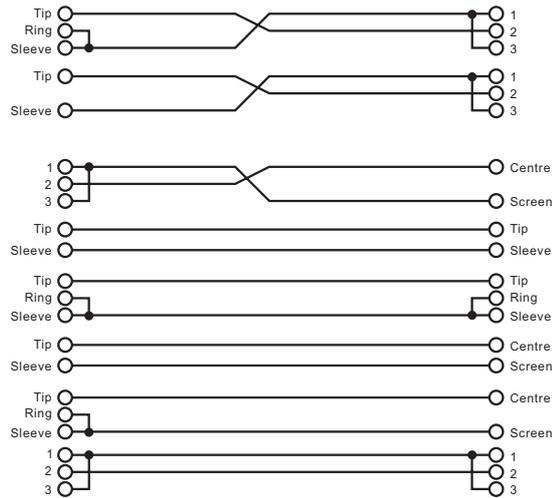
If you are connecting to a mixing console's main inserts, you may have a single TRS jack for Send and Return, in this case, use an insert "Y" cable that configured like the examples below.
