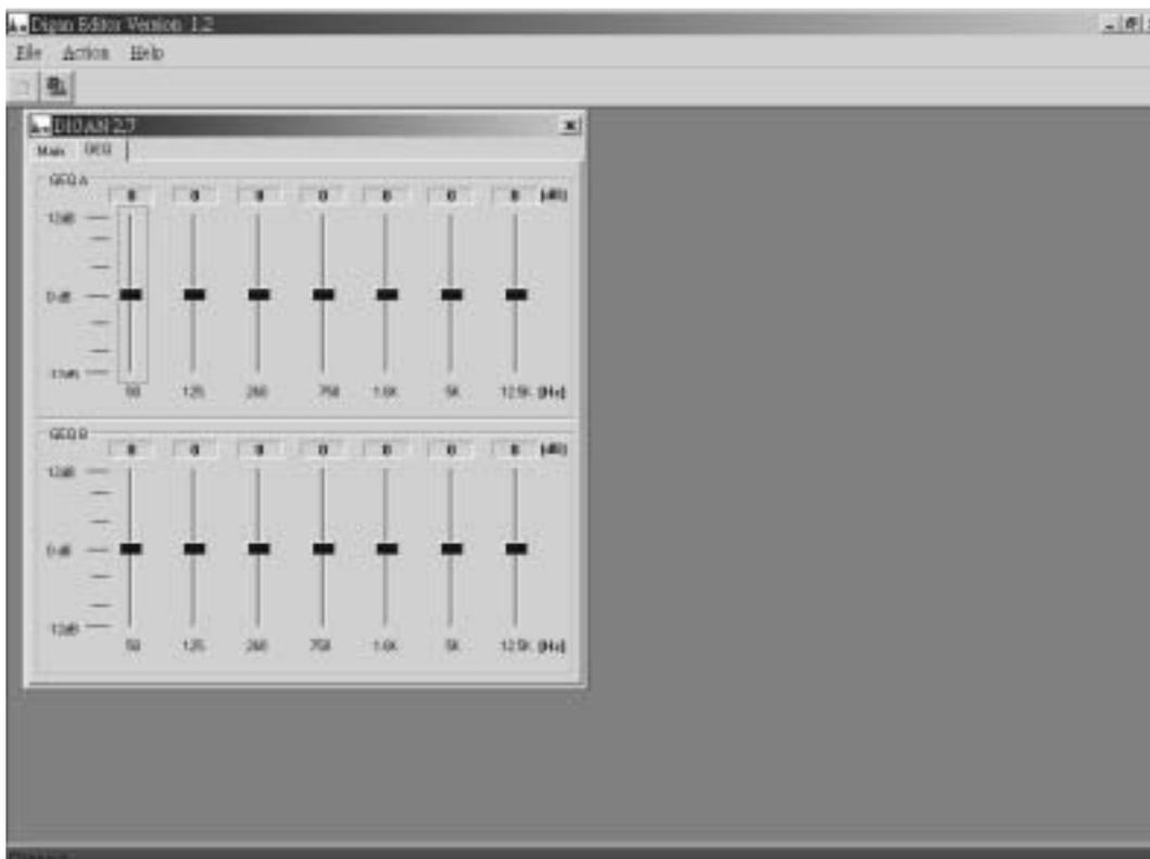
When you go to graphic equalizer, the PC will display above picture. You can adjust each band's gain value, if this unit is in LINK function, the change on channel A will be applied to channel B also. The adjustable range goes from 12dB to +12dB.
