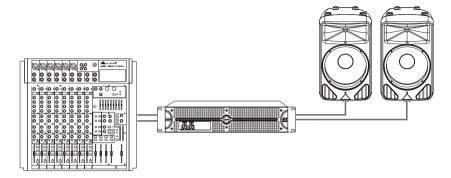
In this mode 2 independent channels are sent to 2 separate speakers.
