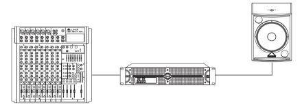
The stereo or mono signal input to CH A and CH B is combined on the BRIDGE MONO connector. Only CH A Gain control is active. The power at the output will be combined power of the two channels.
