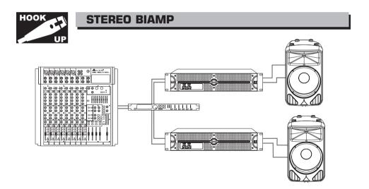
This application is only for D1 or D3. For the D2 or D4, it has four channels so only use one amplifier. The Main Mix signal is routed into an electronic crossover. CH A drives the woofer and CH B drives the high frequency driver in a 2-way enclosure.
