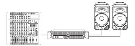
One mono signal is input to  $CH\ A$  or  $CH\ B$  of the D series amplifier and then output to 2 separate speakers. Each speaker volume can be set separately.
