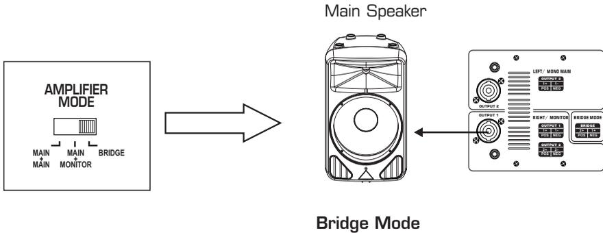
With the AMPLIFIER MODE switch in BRIDGE position, the two power amplifiers in your PBM8 drive together a single speaker cabinet with the sum of the power of the 2 amps. Usually this solution is used to drive a single subwoofer and the MAIN OUT output on the front panel are used to feed a pair of powered speakers as mid-high units.
