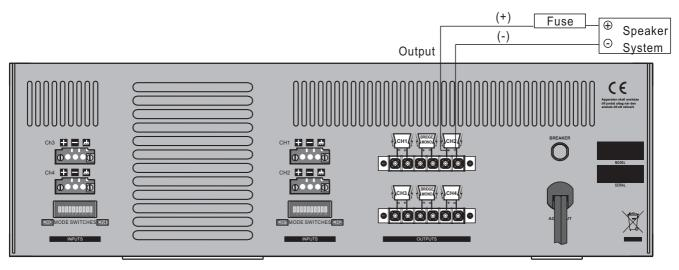
Use the following formula to determine the fuse capacity according to the speaker's input capacity.
