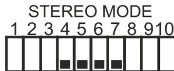
**Parallel mode:** turn these small dip switches of 4, 5, 6, to the top, and turn the small dip switch of 7 down, then channel 1 and channel 2 are in parallel mode.
