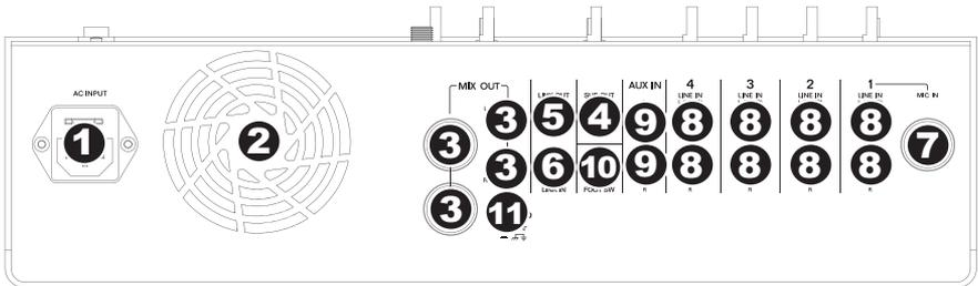
1. **POWER INPUT** – Connect the included power cable to this input and connect the other end of the cable to a power source. Make sure the top panel's POWER SWITCH is set to "off" when plugging and unplugging the cable.
