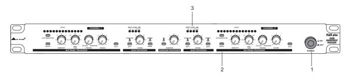
Your ▲LTO FLEX plus presents with surround processor and two identical channels, and each channel is equipped with the multi-band processor and bass processor, which contains 5 push-button switches, 5 rotary controls and 17 LEDs.
