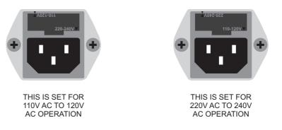
The fuse-holder above the AC connector on the rear of the chassis has 3 triangular markers(please refer to the above pictures), with two of these triangles opposing each other, your unit is set to the operating voltage printed next to these markers.
